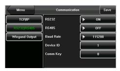
**RS232:** This parameter is used to enable or disable the RS232 communication. If the RS232 communication cables are used, set this parameter to "ON".
