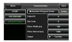
**Wiegand Format:** The system has two built-in formats **Wiegand 26-bits** and **Wiegand 34-bits**, and also supports the format customization function to meet individualized requirements.
