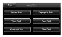
**Screen Test**: The IFACE terminal automatically tests the display effect of the color TFT display by displaying full color, pure white and pure black and checks whether the screen displays properly. You can continue the test by touching the screen or exit it by pressing [Auto Test].
